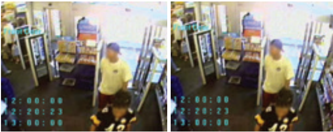
Video with correct aspect ratio (L); video that has been vertically stretched (R). The image on the right makes the subject look thinner than he really is.
